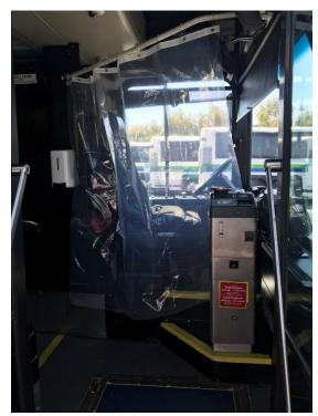
The picture above is an example of the driver barrier (in the "deployed" position) and the hand sanitizing station
