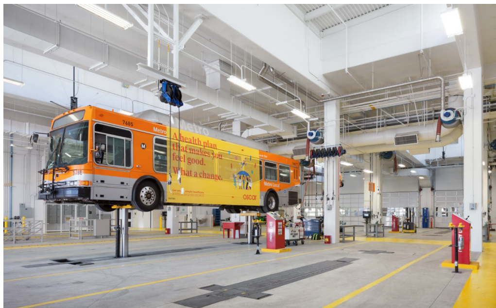
Drive-Through Maintenance Bay with In-Ground Vehicle Lift (LA Metro Division 13 Bus OMF, Los Angeles, CA)
