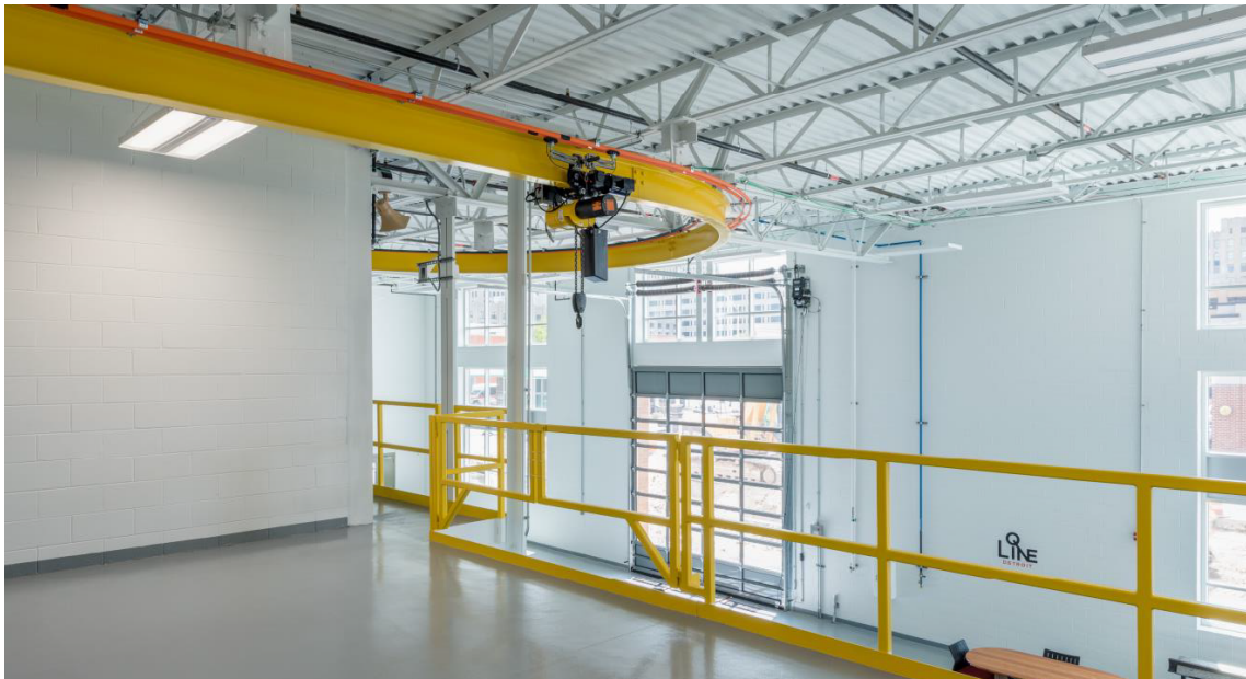
Typical Mezzanine Storage with Monorail Crane and Swing Gates (Q-Line Streetcar Vehicle Maintenance Shop, Detroit, MI)
